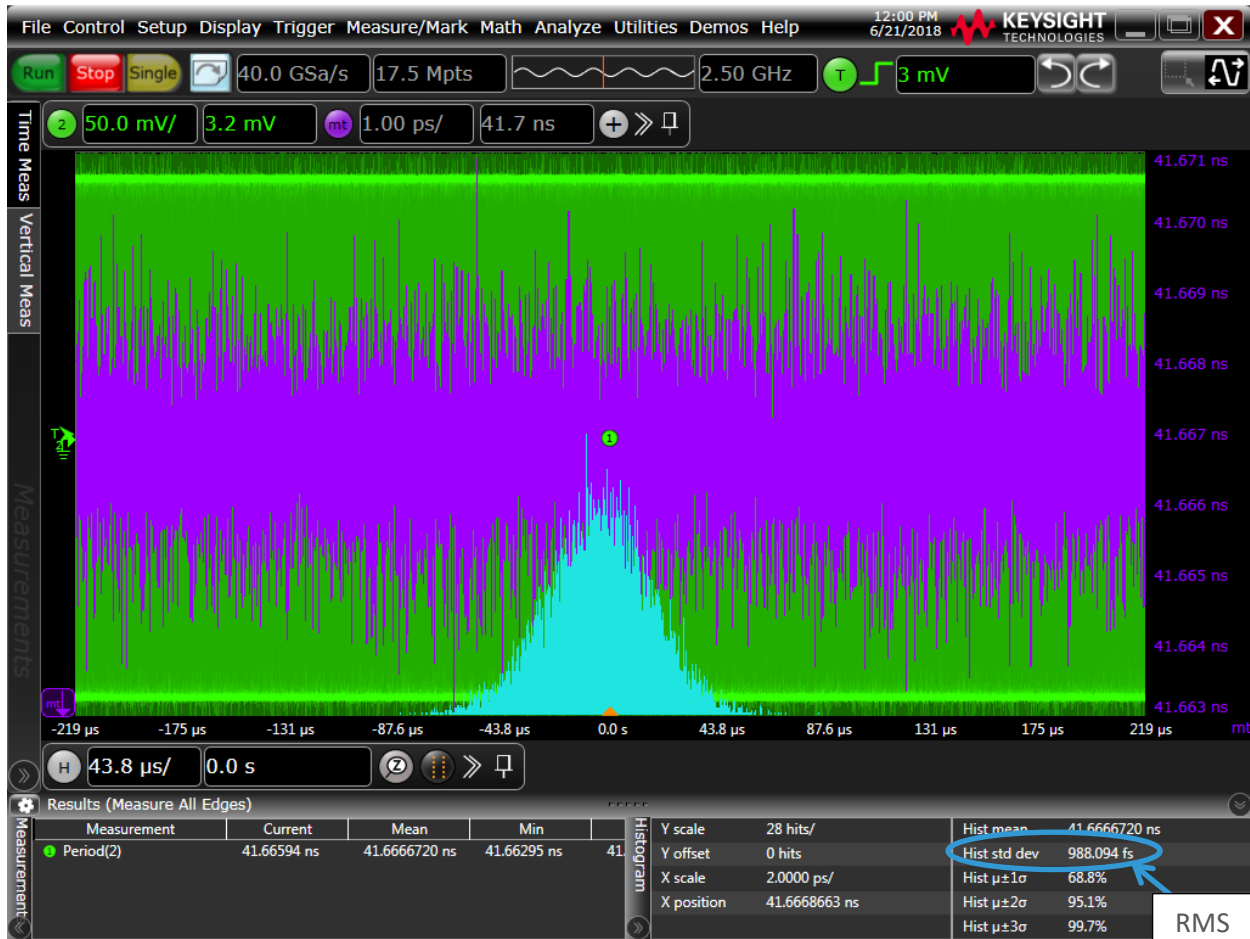
Figure 3. Period jitter screenshot of 10,000 period jitter measurements
